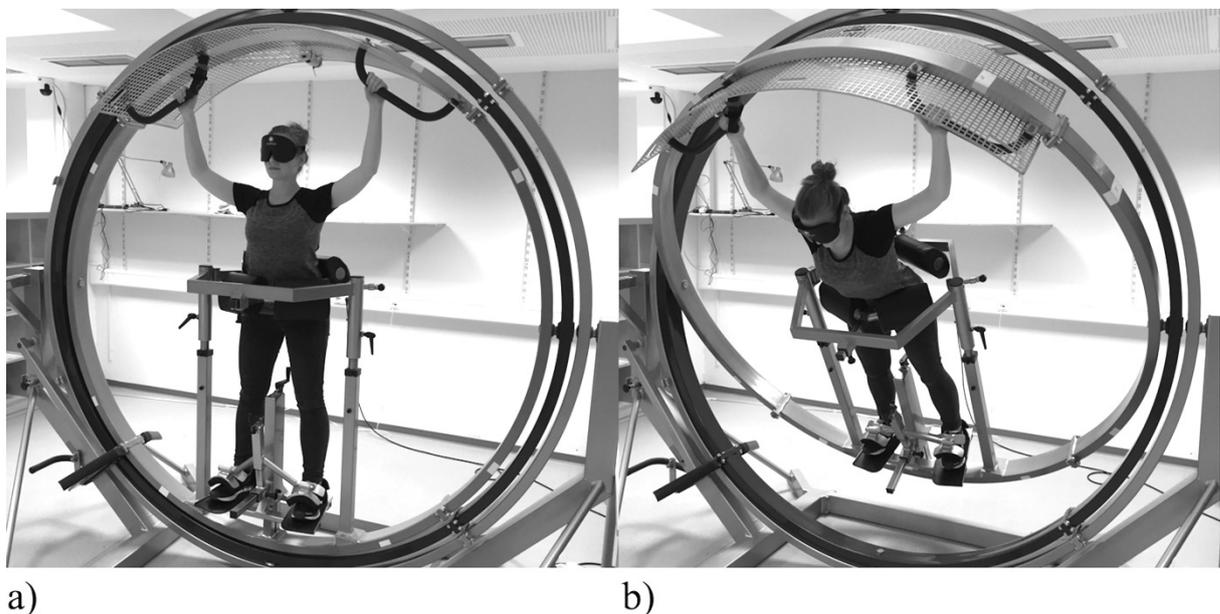
*Figure 1.* SpaceCurl human gyroscope with a participant in vertical position (a), and in forward rotated orientation (b). The gymnast is wearing the Mindfold® mask. The gyroscope sensor is attached to the top of the inner ring of the gyroscope.
